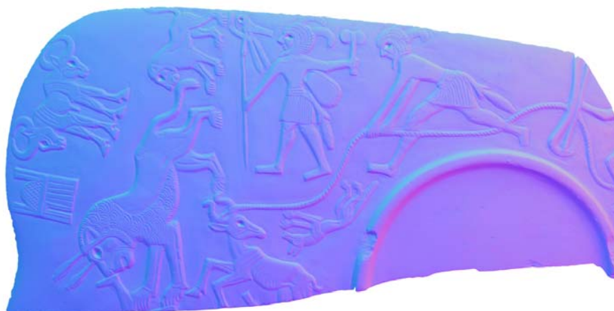
Surface normals of the Hunter's Palette, derived by the photometric stereo method, shown in false colour with the X,Y,Z components represented by R,G,B channels.
