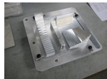
Figure 6. The 3D Geometric target plate including: step artefact; gap artefact; angle artefact and length control. At this pre-assembly stage surface treatments have not yet been applied.
