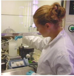
Figure 7. Surface treatment by alkaline etching in the lab: suspending the test cubes in the sodium hydroxide solution.
