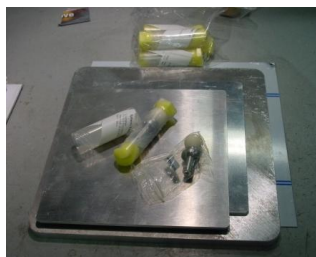
Figure 2. Inset plates with the calibrated tooling balls during the manufacturing process.
