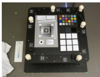
Figure 5. The completed 2D photographic target plate: Left ISO-16067-1 chart to test resolving power, top right: x-rite colour chart, bottom right: gloss scale.
