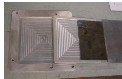
Figure 3. Milled base plate during the manufacturing process. From left to right: base plate with hole for the spheres; artefact base with steel base next to it; 2D base plate.
