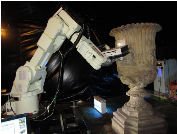
Figure 7. The measurement system during digitisation of the first vase.
