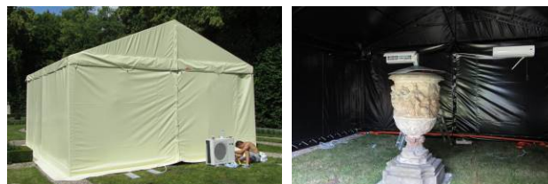
Figure 6. The tent covering the object and measurement system during digitisation.
