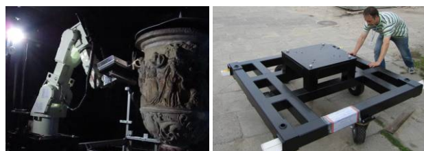
Figure 5. Positioning devices: a) Kawasaki FS20N robotic arm, b) Platform for the robot arm.
